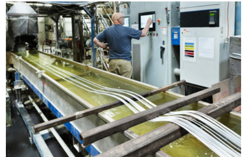
Extruded engineered thermoplastics are cooled and pelletized.
