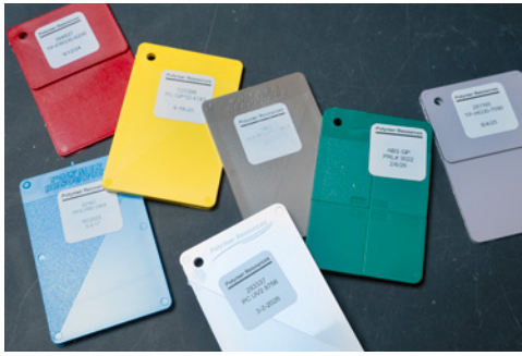
Color quality is validated with both a spectrophotometer and by visual inspection.
