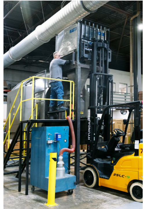
The hopper is forklifted above the Rotary Batch Mixer inlet where the contents are discharged via a knife gate into the mixer as it rotates.
