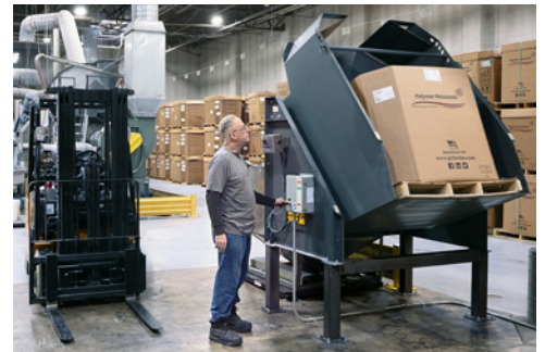
A box dumper unloads the contents of each container into a portable stainless steel hopper.
