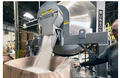
Internal flights direct blended material toward and through a plug gate valve with no stratification into a Gaylord on a scale.
